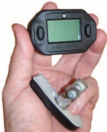
Tire Watch Display and Internal Sensor
