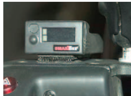
SmarTire Display Mounted on BMW Clutch Reservoir
